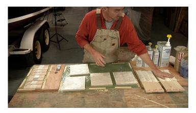
For my experiment I decided to focus on 3 common factors that come into play when doing repair work; Fine edge bonding, flexing stress, and shear strengths. All of these tests were done comparing the three West System hardeners I commonly use with their 105 resin; 205 fast hardener, 206 slow hardener and 207 special clear hardener. The glass used for all the tests was 1708 Bi-axial.
